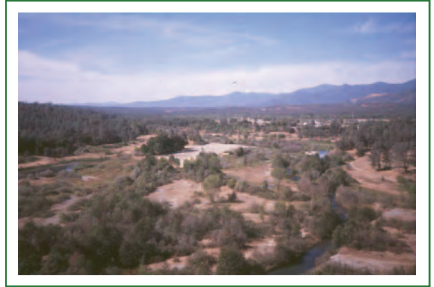
Above: Phase One completed. The plug area (center of photo) was put into place to prevent salmon and steelhead from reaching the pond (left side of photo) during high water and getting stranded after flows subside. • Source: Western Shasta RCD
