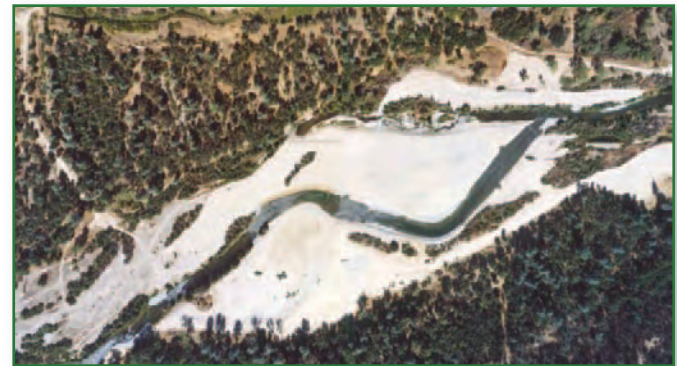
Above: The Western Shasta RCD redirected the Creek into the cobble-bedded channel that provides much better spawning habitat for fish.
